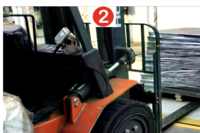
HOLI indicator fixed in the cabin of forklift truck
